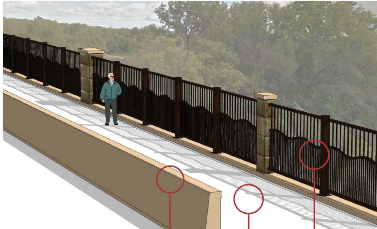
Figure 2.15 Ornamental Wave Railing
